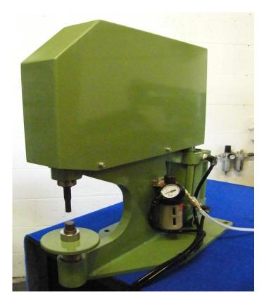
The pneumatic cylinder mounted at the rear of the head is connected to the downward moving punch holder by a simple leverage system, giving a riveting stroke of 20mm. The foot pedal can be located from either left or right foot operation.
